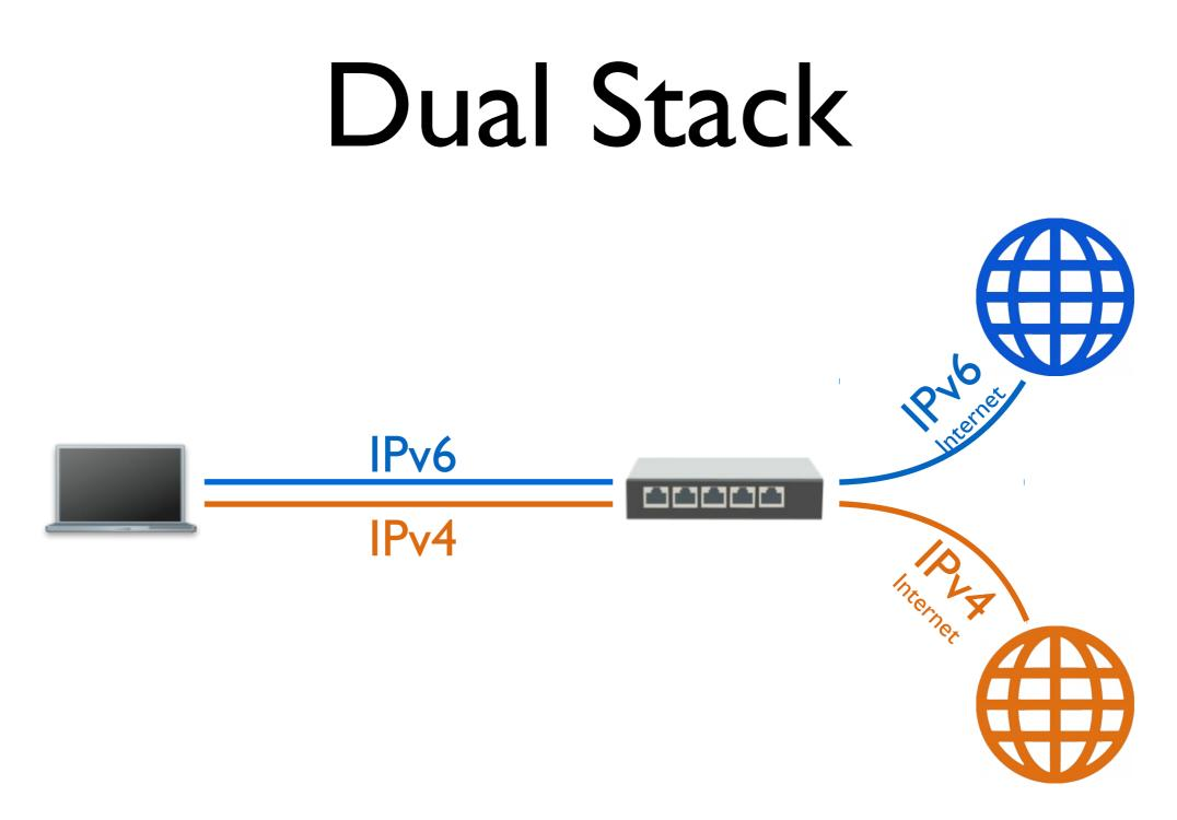
End-user device (host) has both IPv4 and IPv6 connectivity
